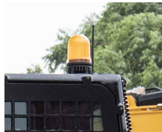
ROTATING WARNING LIGHT: It always reminds people around to maintain a safe distance.
